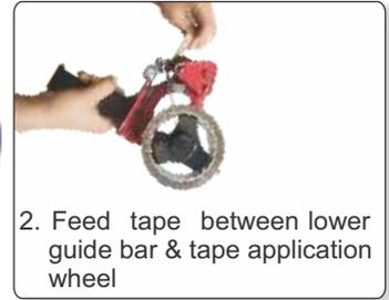
2. Feed tape between lower guide bar & tape application wheel
